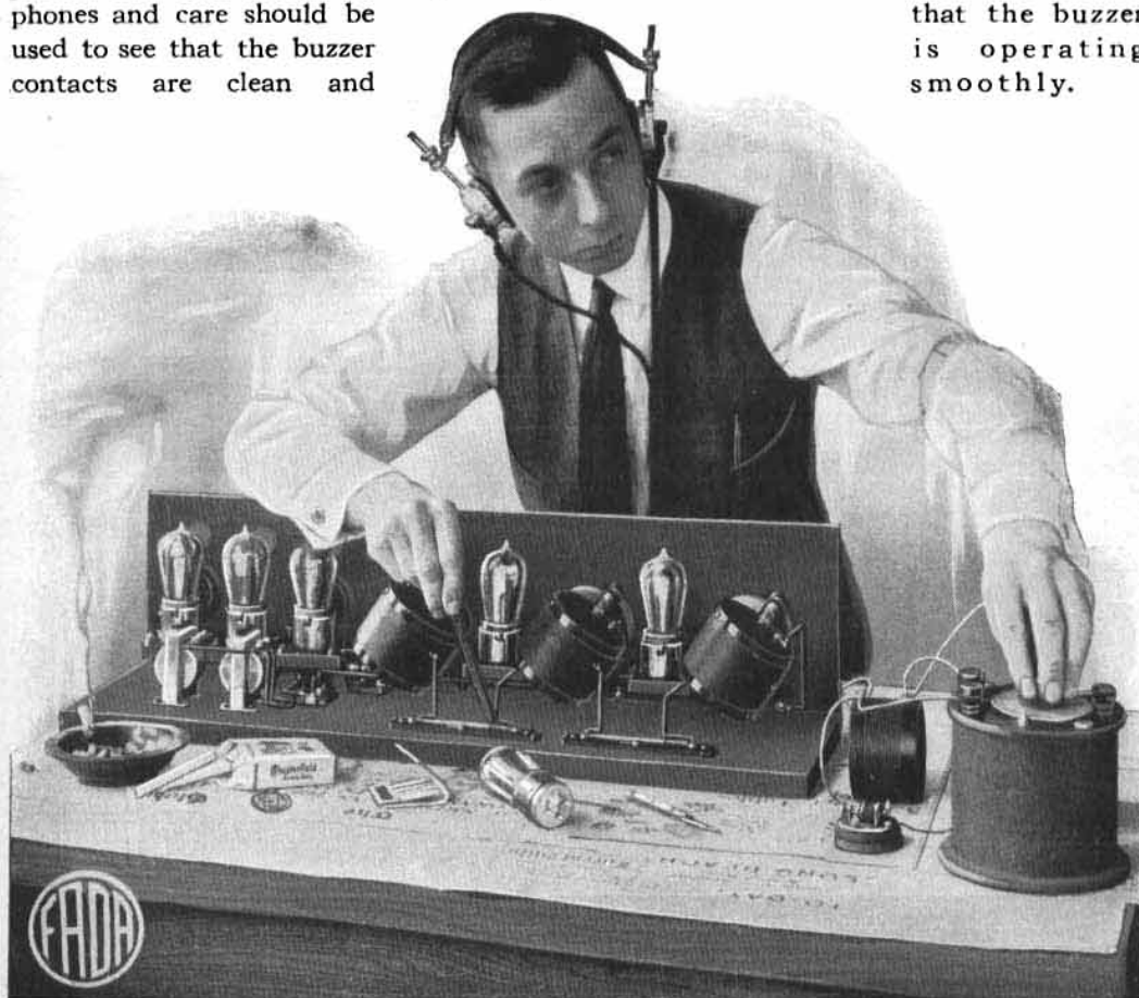
Showing the five tube "Neutrodyne" receiver being adjusted for complete neutralization.
