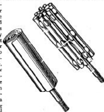
Fig. 50.—Two typical anode designs used in electrolytics.
