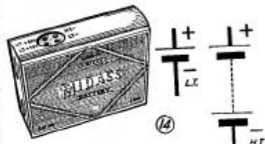
Fig. 11.—The theoretical signs for low tension (L.T.) and high tension (H.T.) batteries. Note that the thin line always represents the positive terminal, and the thick line the negative terminal. On the left is a pictorial view of an all-dry combined L.T. and H.T. battery, but in most cases the accumulator is of the wet type: that is to say it contains dilute sulphuric acid and can be recharged.
