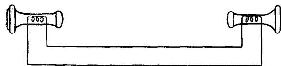
FIG. 9-4 ELEMENTARY TELEPHONE CIRCUIT
