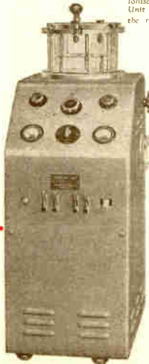
903A Oil Diffusion Pump with combination baffle valve. Peak un baffled and baffled speeds... 1500 and 900 litres/second respectively.
