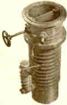
903A Oil Diffusion Pump with combination baffle valve. Peak un baffled and baffled speeds... 1500 and 900 litres/second respectively.
